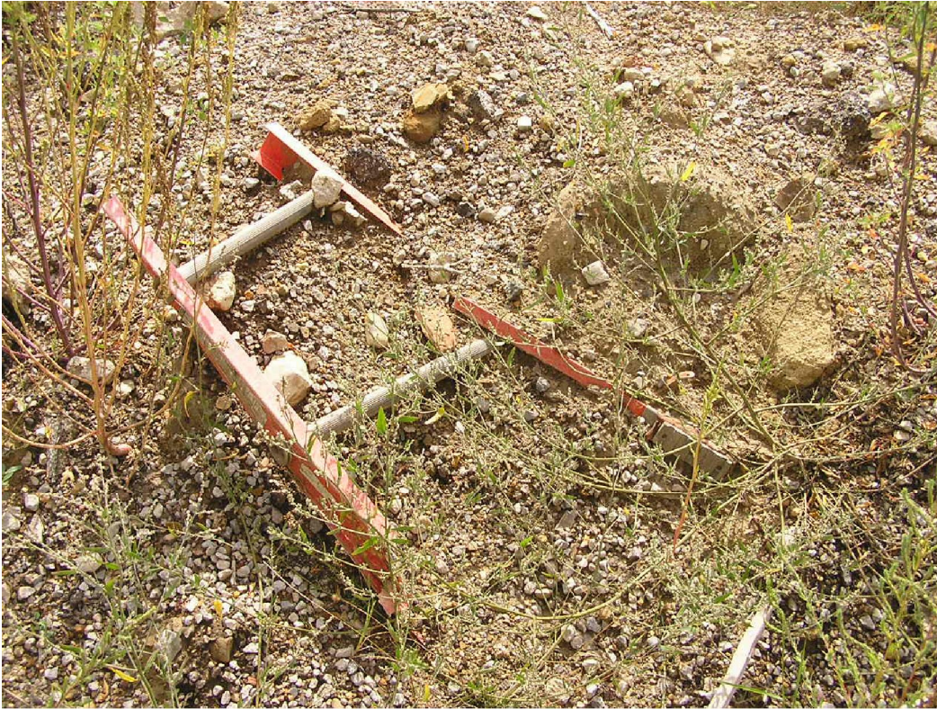
Date:09-04-2014 Time: 12:33PM Direction: Southwest Photo by: Jen O'Hearn Exposure #: 007 Comments: View of a broken fiberglass and metal ladder.
