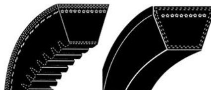
Figure 4: Notched Belt (left) and Standard Smooth Belt (right) 3
